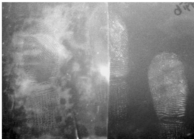
Fig. 6 Three-week-old fingerprints on polyethylene, developed using powdering (left) and SPR (right); illumination at 350 nm and detection using a 570 nm long-pass filter
