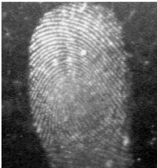
Fig. 5 A 10-day-old fingerprint on glass developed with nanostructured ZnO using the powder and brush technique and detected using a 570 nm long-pass filter with 350 nm illumination
